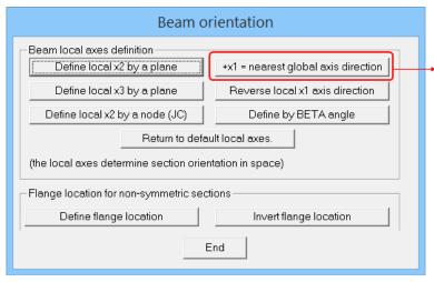
The local x1 axis is always parallel to the axis of the beam. Revise +x1 so that it points in the general direction of the closest positive global axis.
