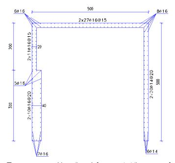
The program combines the reinforcement at the corners from attached segments:
