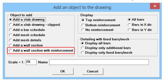
This option creates a wall cross section drawing with reinforcement. The program currently draws only the vertical reinforcement. For example:
